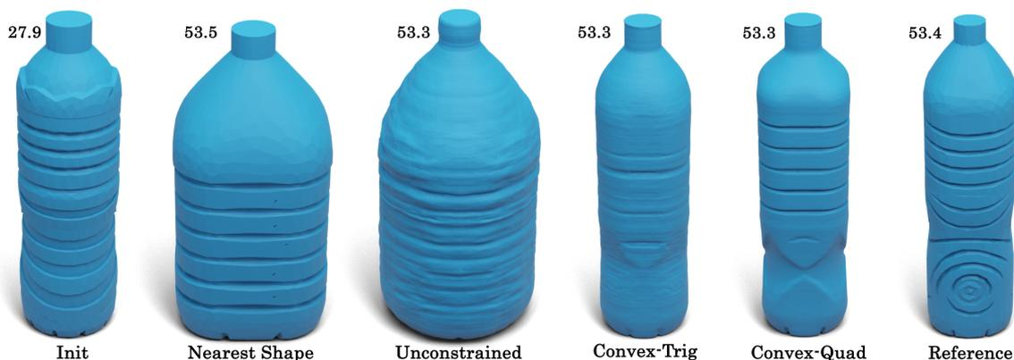
Figure 1: Illustration of our approach. Given an initial shape and a target topload value (53.3 annotated), we would like to find a shape for this prescribed topload (right-most). Unconstrained optimization produces a shape with significant change in the volume while optimizing in the convex neighborhood yields a more realistic shape. Ours, which optimizes in the convex-hull of a quadrilateral produces the most plausible result.
