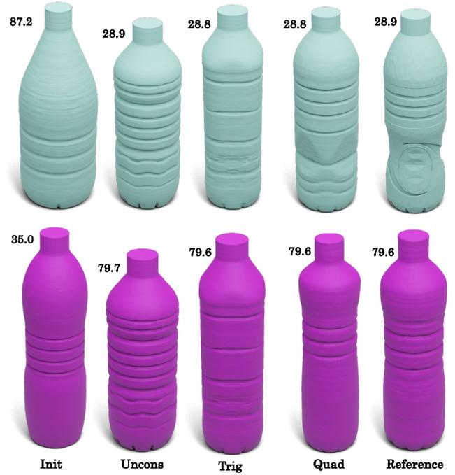
Figure 9: Comparison of different techniques for optimizing the starting shape (left-most column) to match query topload. The initial shape is chosen such that its topload is furthest from the target topload. First row shows a case where we reduce the topload while the second row shows a case where topload is increased. Note that unconstrained produces a similar shape in both cases.
