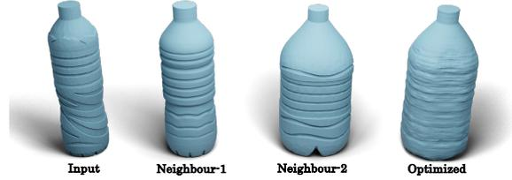
Figure 7: Illustrating the non-convergence issue due to drastic change in volume of the initial shape. Due to a sub-optimal choice of neighbor, our convex-space optimization results in an optimized shape (third column) that bears a significant volume increase.
